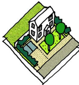
On-plot parking on driveway
